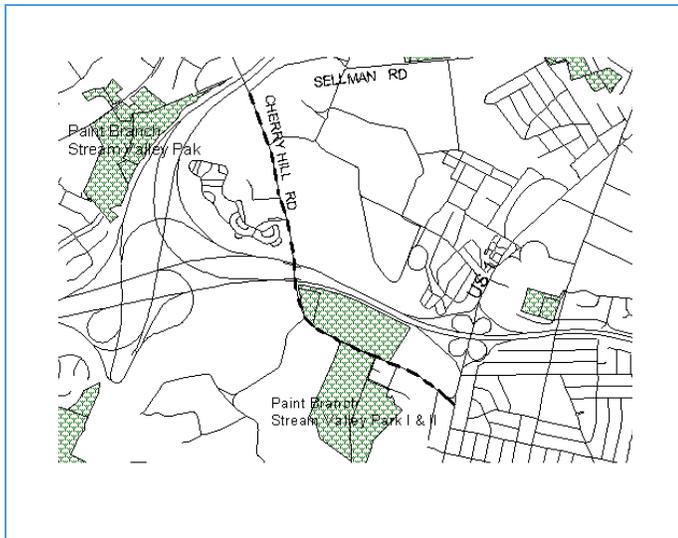
**Description:** This project reconstructs 1.6 miles of Cherry Hill Road from Sellman Road to Little Paint Branch, north of US Route 1. It also includes widening two bridges and replacing one. The project will reconstruct the existing two-lane roadway to provide additional traffic lanes. Also included are bike trails, sidewalks, additional traffic signals and street lighting.
