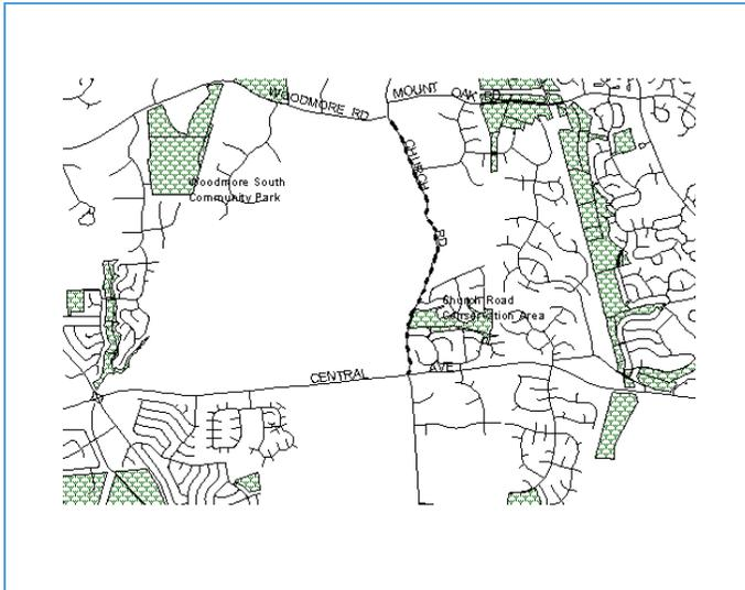
**Description:** This project provides geometric and safety improvements to Church Road between Woodmore Road and MD 214 (Central Avenue). Improvements will include intersection improvements, local realignment of the roadway as well as the addition of shoulders and roadside drainage where necessary. The horizontal and vertical alignment of the roadway will be improved.
