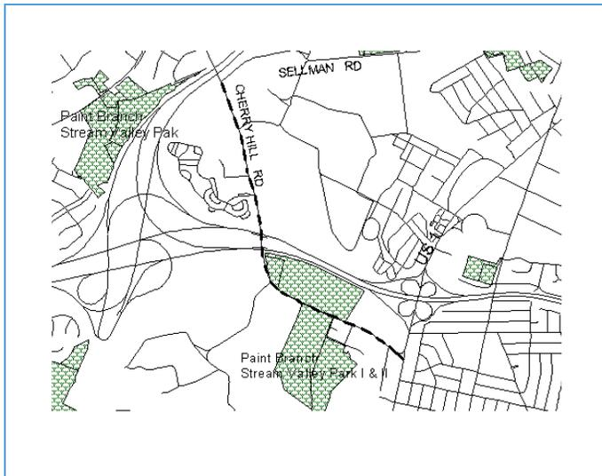
**Description:** This project reconstructs 1.6 miles of Cherry Hill Road from Sellman Road to Little Paint Branch, north of US Route 1, and includes widening two bridges and replacing one. The project will reconstruct the existing two-lane roadway to provide additional traffic lanes. Also included are bike trails, sidewalks, additional traffic signals and street lighting.
