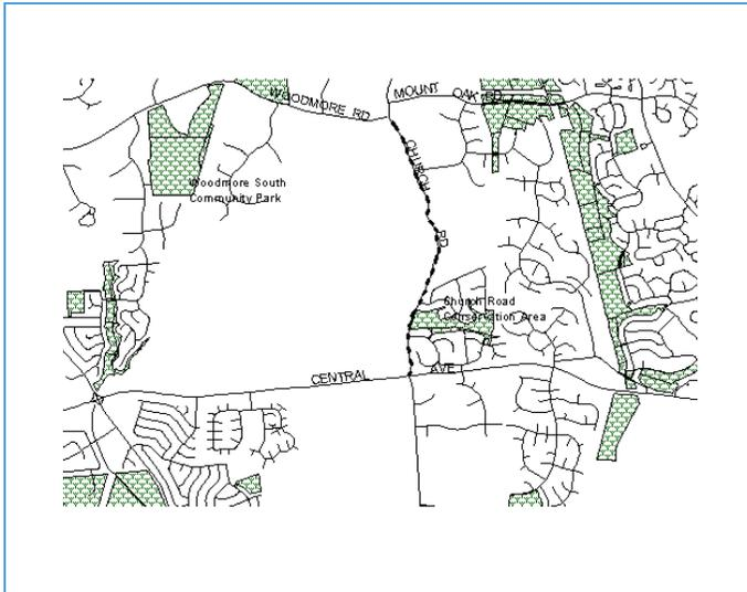
**Description:** This project provides geometric and safety improvements to Church Road between Woodmore Road and MD 214 (Central Avenue). Improvements will include intersection improvements, local realignment of the roadway, and the addition of shoulders and roadside drainage where necessary. The horizontal and vertical alignment of the roadway will be improved.
