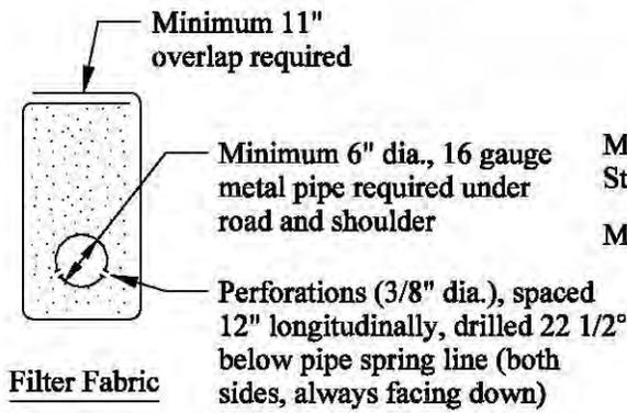
Filter medium allows water to pass through while preventing soil particles from migrating into drainage stone.
