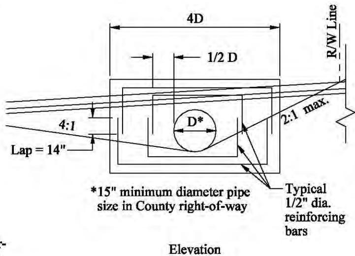
\*15" minimum diameter pipe size in County right-of-way
