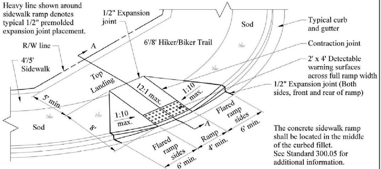
The concrete sidewalk ramp shall be located in the middle of the curbed fillet. See Standard 300.05 for additional information.
