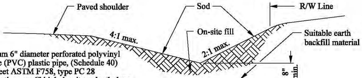
Minimum 6" diameter perforated polyvinyl chloride (PVC) plastic pipe, (Schedule 40) shall meet ASTM F758, type PC 28 specifications, or 6" high density polyethylene (HDPE) plastic pipe shall meet AASHTO M 294 specifications and include 50 psi minimum stiffness. Minimum 6" dia., 16 gauge perforated metal underdrain pipe required under roadway and shoulder.
