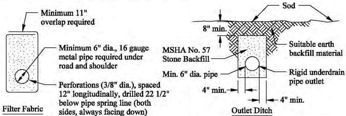
Filter medium allows water to pass through while preventing soil particles from migrating into drainage stone.
