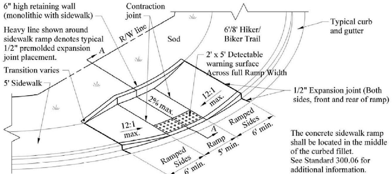
The concrete sidewalk ramp shall be located in the middle of the curbed fillet. See Standard 300.06 for additional information.
