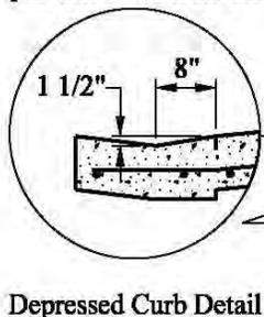
Depressed curb to have two (2) No. 4 (1/2" dia.) longitudinal reinforcing bars parallel to roadway.
