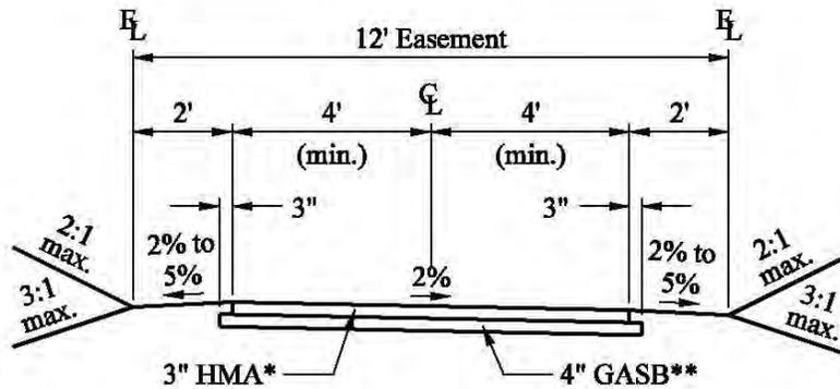
\*3" Hot Mix Asphalt (HMA) surface (fine gradation only). For criteria see Section II, "Technical Specifications."
