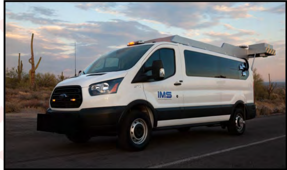
Pavement Survey Vehicle
